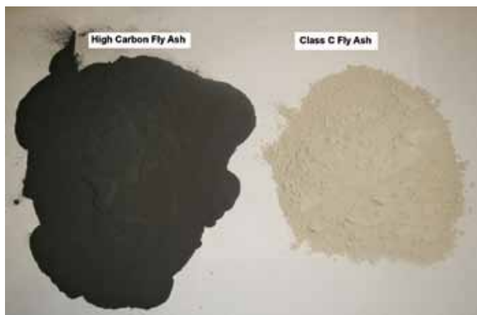
Unlike buff-colored conventional Class C fly ash (right), the dark color of HCFA has been a barrier to beneficial use in concrete (photo courtesy of We Energies)
