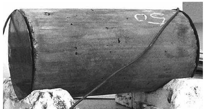
A cylinder of electrically conductive HCC, with electrodes on either end, is tested for conductivity (photo courtesy of We Energies)
